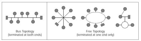
The individual users are connected one after the other in parallel with bus topology. The bus must be terminated at the beginning, and at the end. Wiring with free topology necessitates only one bus terminator, although it is restricted as regards maximum transmission distance.
